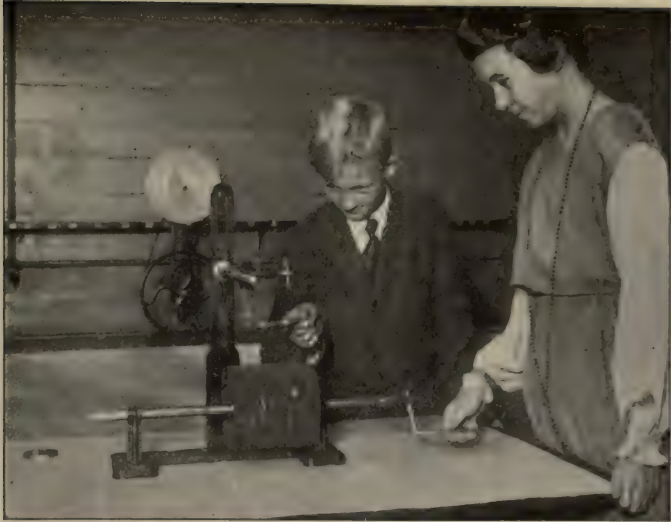
FIG. 101. When the tuning fork vibrates, the glass needle makes a wavy line on the smoked paper on the drum.
